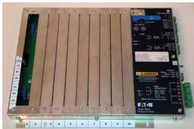
Figure 36. Cover Plate Removed from Slot 1.
