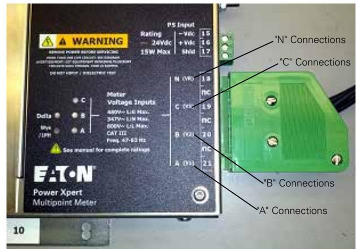
Figure 8. A, B, C, and N Connections on the PXMP-MB Assembly Meter Voltage Input.
