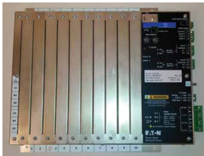
Figure 35. Removing the Mounting Hardware and Cover Plate.
