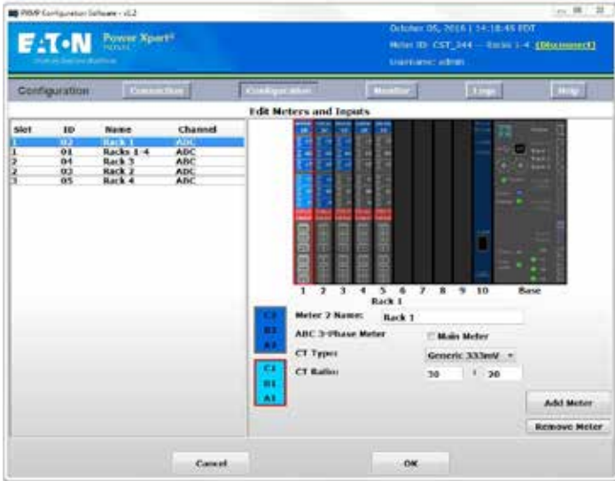
Figure 29. New Configuration Screen - Used to Enter Information for Each Slot in the Meter Base.
