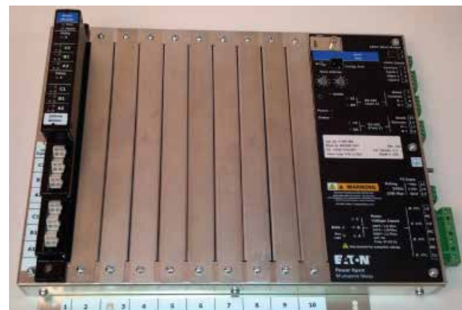
Figure 37. Module Installed in the Meter Base Assembly.
