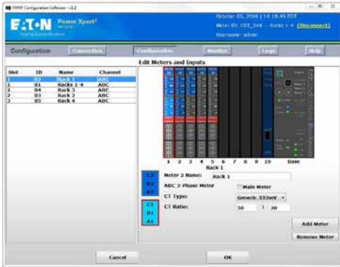
Figure 28. PXMP Configuration Software Meter Configuration Screen.
