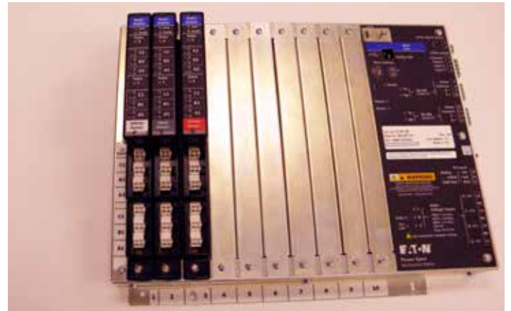
Figure 5. PXMP-MB Assembly Components and LEDs.
