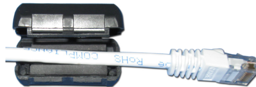
Figure 2. cable placed in bead
