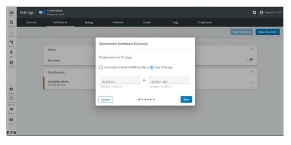
• When a device stops communicating or has a communication issue, it is difficult to pinpoint the problem. Dashboard Campus now has a diagnostic capability for troubleshooting in case of communication or navigation failure to downstream dashboards.
