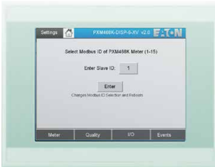
Figure 7. Changing the Modbus ID.
