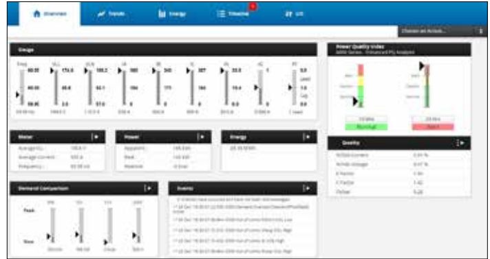
Figure 13. Main Screen of Meter Interface.
