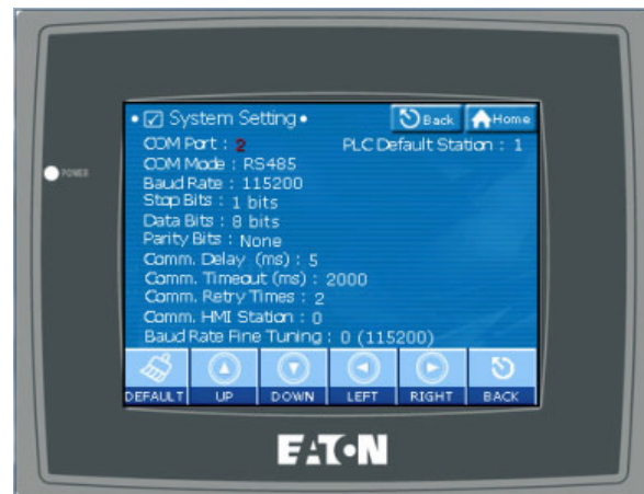
Figure 6. Changing the PLC Default Station.
