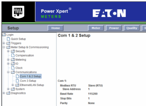
Figure 5. Meter Web Server Configuration Screen Com 1 & 2 Setup.
