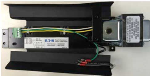
Figure 13. PRCEPP Power Supply
