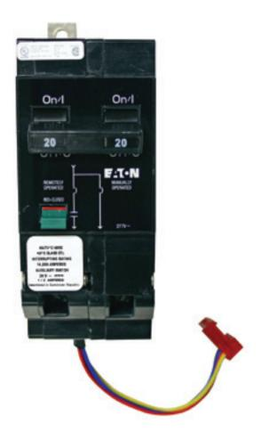
The GHQRSPEL circuit breakers contains both a solenoid operated remote switching circuit and a manually operated thermal-magnetic circuit breaker. This Emergency Lighting Circuit Breaker complies with the 2008 National Electric Code; Section 700.12(F) for Sources of Power utilized in emergency lighting applications.
