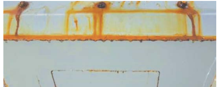
Generic steel enclosure after 1200-hour salt spray
