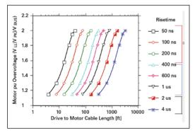
Figure 1. Cable Length Versus Overvoltage [2]
