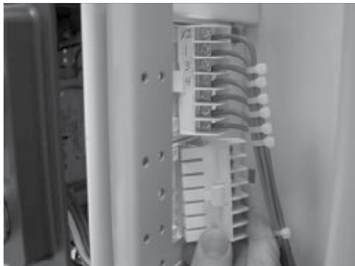
Figure 29. Disengaging pull-apart terminal blocks
