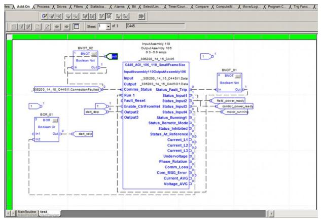
Fig. 5 Typical function block of the motor management relay showing inputs and outputs assigned to the PLC program
