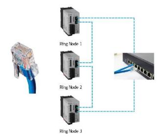
Fig. 2 At left, a typical RJ45 Ethernet connector used with standard Cat 5 cable media. At right, Device Level Ring Ethernet topology
