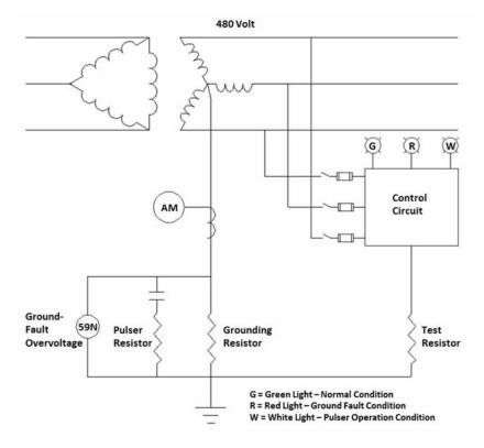
Fig. 8 Low-Voltage pulsing high-resistance ground system
