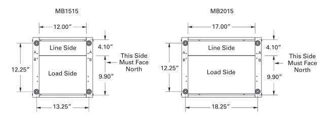
Method 2. Use anchor bolts (5/8" dia.) pre-cast in concrete pad. Mounting hole dimensions are shown above for MB1515 ( $15'' \times 15''$ ) and MB2015 ( $20'' \times 15''$ ) pedestals. Locate line and load conduits the same as in Method 1.
