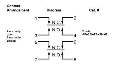
Figure 3 • Switch Contact Arrangement
