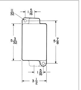
Note: Depth is 5.5" from front of switch to back of box.
