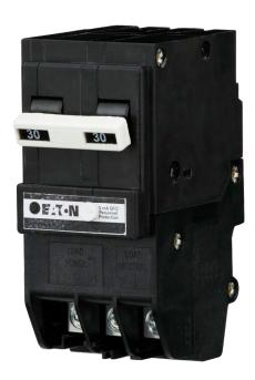
The redesign of Eaton's BR two-pole ground fault circuit breaker yields a new approach to ground fault protection that significantly reduces nuisance tripping events while improving diagnostic speed and resolution of problems. Through its microprocessor-based design, the BR two-pole ground fault circuit breaker makes decisions about leakage and responds appropriately in milliseconds, enabling the circuit breaker to disregard transient conditions that could lead to tripping.
