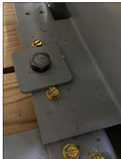
Figure 16. Mounting With Washer.
