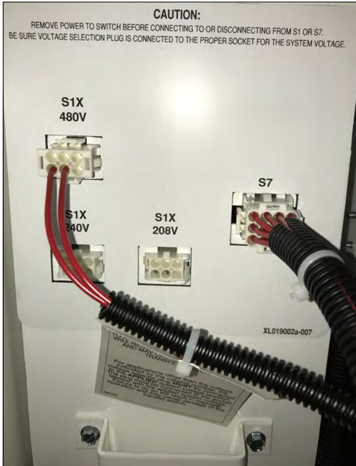
Figure 22. Voltage Selection Adjustment.
