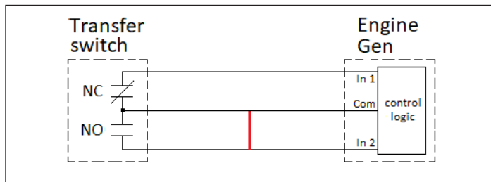
Figure 8. Three-wire start circuit when normal power source is available. Shorted wire condition at NO loop. Identical logical states (closed-closed) sensed by engine-generator control logic inputs
