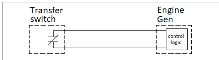
Figure 1. Transfer switch start contact closes signaling an engine start when the normal power source becomes unavailable
