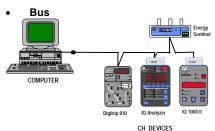
Multiple devices connected on a common wire.
