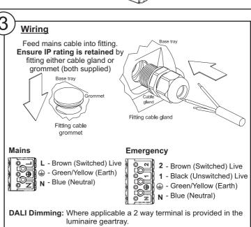
Product suitable for looping with max conductor size 2 x 2.5mm<sup>2</sup>
