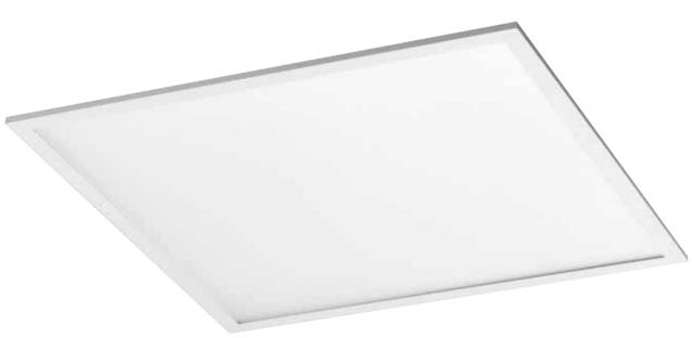
The Modulay LG is a high performance IP20 LED 600x600 flat panel luminaire with a prismatic diffuser to reduce glare and increase visual comfort.
