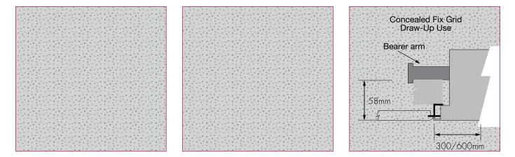
Note: luminaires will typically have 1.5mm clearance between the edge of the luminaire return and the centre line of a ceiling grid system e.g. grid centres 600mm x 600mm luminaire dimensions 597mm x 597mm.
