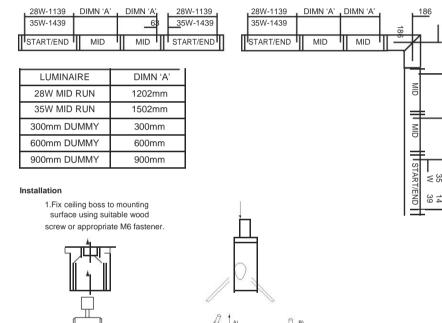
Feed 1.5m long wire into fastener body as shown. Screw body into ceiling boss.
