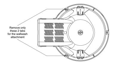
Note:When using any of the attachments apart from the halo glass on emergency luminaires use the LED bracket supplied, hooked over the lamp cutout in the reflector. For the halo glass fit the LED into the bezel as a standard emergency luminaire
