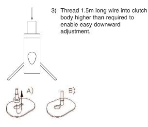
Offer housing up to 'Y' section wire and feed nipple ends into keyhole slots.
