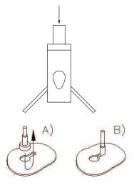
3. Thread 1.5m long wire into clutch body higher than required to enable easy downward adjustment.
