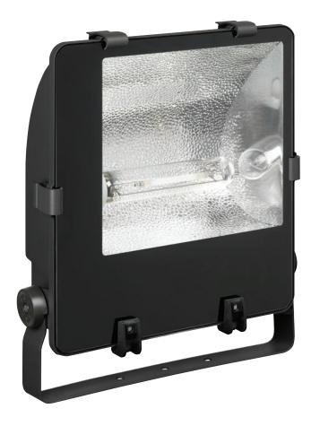
Galaxy Major has been designed with an all new 'floating glass' architectural housing and solves the problem of sky glow and light trespass by employing an asymmetric reflector system. Galaxy Major is rated to IP65, dust tight and low pressure water jet proof, with a robust die-cast aluminium body providing a long and reliable service.
