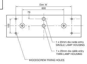
Note: Luminaire housing must be mounted direct on to ceiling surface, they are NOT suitable for suspension or trunking mounting.
