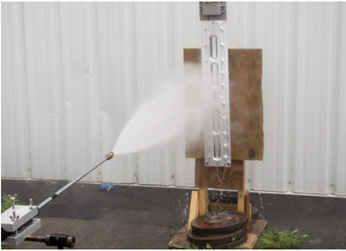
Pauluhn ZPL tested to withstand 2,000 psi hose test at 5 ft. distance
