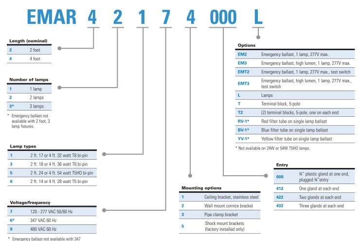
VAC model, 2 ft. fixtures or 4 ft. fixtures with wall bracket.
