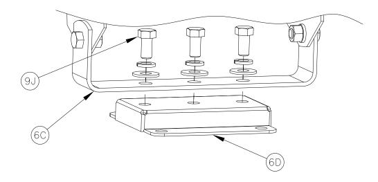
3. Aim the fixture. Loosen the two bolts (9I) holding the 'U' bracket (6C) to the fixture. Rotate the fixture to the desired direction and securely tighten the 'U' bracket bolts (9I).
