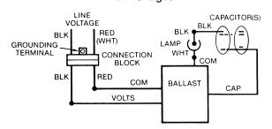
**High Pressure Sodium (HPS)** — 50, 70, 100 and 150 watts 208, 240, 277, 480 volts
