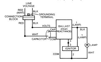
High Pressure Sodium (HPS) — 200, 250 and 310 watts
