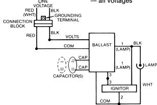
High Pressure Sodium (HPS) — 400 watts — all voltages
