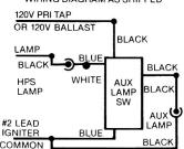
100 watt maximum in fixture with suffix QTZ (quartz)
