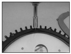
Break seal between gasket and housing. This can be difficult depending on the amount of time the fixture was in service.
