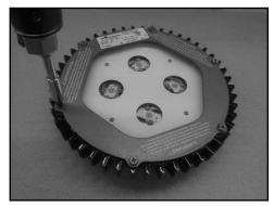
Insert flat head screwdriver between gasket and lens, being careful not to damage gasket.
