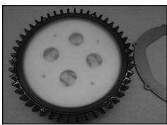
9. Reinstall lens retaining bezel; torque to 30  $\pm$  3 lb.-in. (2.26  $\pm$  0.3 N-m).
