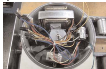
Figure 7. Complete Luminaire Assembly (plastic cover not shown)
