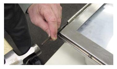
2. With pliers, pull the hinge-pin completely out, releasing the door.
