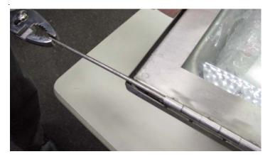
Replace with the new door, inserting the new hinge-pin all the way through the door hinges.
