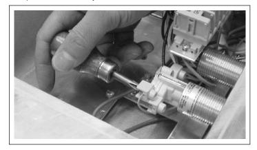
b) Remove wire tie and disconnect wire nuts attaching one (1) black and one (1) white wire lead from the indicating pilot light to the circuit board.
