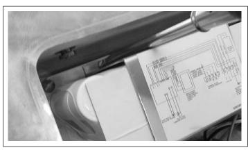
Loosen the lower two (2) screws holding the battery bracket and remove battery and bracket.
