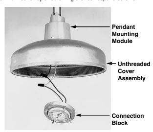
3. Apply a small amount of HTL® Lubricant to threads. Thread cover into module until mounting module seats firmly against O-ring seal and secure with set screw.
