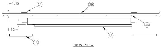
3) Lateral position between fixture mounting joist (2A) and Ceiling System Track Clip (3C) is critcal.
