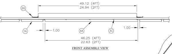
4) Ceiling Panel (1A) will cover opening (5A) betweeen lens frame and fixture housing (see figure 1 and figure 2).
