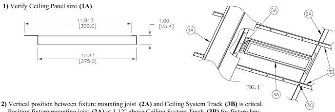
2) Vertical position between fixture mounting joist (2A) and Ceiling System Track (3B) is critical. Position fixture mounting joist (2A) at 1.12" above Ceiling System Track (3B) for fixture lens frame (4A) to be flush with Ceiling Panel surface (1A).
