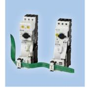
The PKE is a motor-protective and system circuit breaker with modular trip blocks; its overload protection is implemented electronically. The two-component motor starter, consisting of a DILM contactor and a PKE motor-protective circuit breaker, is suitable for simple component replacement using plug-in connection technology up to a rated current of 15 A.
