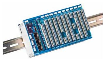
A wide range of functions and interfaces enable the flexible use of the compact, high-performance control system in modular automation solutions. Ethernet interfaces for connection to different networks, along with the standard CAN and RS485 interfaces, turn the XC300 device into a universal control and communication point within the networked facility.
