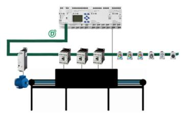
Variable frequency drive: The easyE4 can be used to set the cycle time and to convert it into a motor frequency. The control relay also monitors errors and prevents conveyor belt failure (e.g. failure due to jammed objects).
