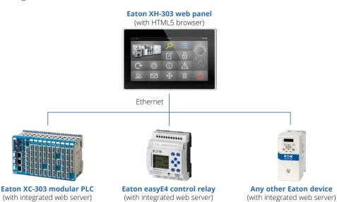
The latter is particularly interesting if, for example, the modular controllers of the XC series or the easyE4 control relay from Eaton are used: They are simply connected to the XH300 web panel via Ethernet and can then display the operating data or the web visualization directly.
