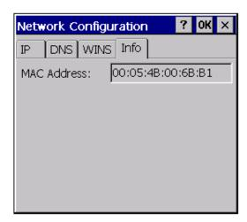
The MAC address of the HMI device is displayed in the Info page. This is a manufacturer-specific and unique Ethernet connection number of the device.
