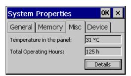
The «Misc» tab displays the current temperature on the device and the operating hours.
