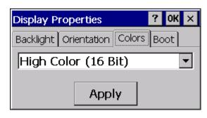
This setting enables the number of screen colors to be selected. Different color depths can be selected. The setting is not transferred until after a restart.
