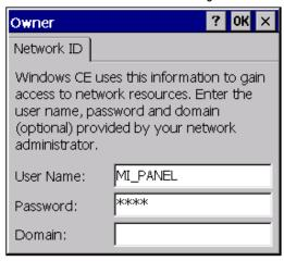
Specific operations must be carried out in order for the selected settings to be retained after a restart. If the entries are acknowledged with OK, the current settings can be saved inside the registry file NETWORK.REG. The content of the REG file must be inserted in the <a href="Autoexec.reg">Autoexec.reg</a> file so that the settings are reset after a restart.
