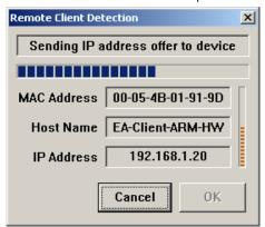
By pressing the OK button, the connection to the device will be established.
