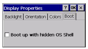
This setting can be used to modify the startup behavior of the device. If this option is enabled, either the <u>Autoexec.bmp</u> bitmap or a black screen will be displayed during startup instead of the Windows CE interface. The execution of the <u>Autoexec.bat</u> file is also not visible.
