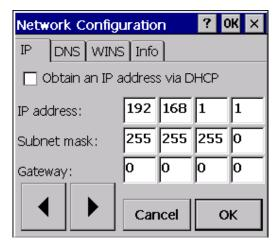
It is always possible for the device to obtain an IP address (network address) via a DHCP server on startup **«Obtain an IP address via DHCP»**. However, for the device to have a unique ID, you should select **«Specify an IP address»**.
