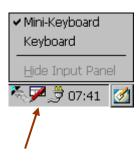
A range of different software keyboards are provided for entering characters on the device. The **«Input Panel active»** setting can be used to activate or deactivate the software keyboard. The option is deactivated by default. A change of this setting requires the system to be restarted.
