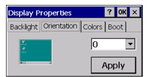
Display orientation can be set with the «0» (default setting) or «90» settings. The display is rotated in a clockwise direction. The «90» setting should be selected for vertical mounting. The picture on the left of the dialog shows the orientation set. The setting is not transferred until after a restart.
