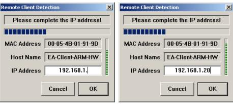
After pressing the OK button the IP address is assigned to the device on the next DHCP request from the device. The "RemoteClient DHCP server" waits for a confirmation from the device that the received IP address has been accepted.
