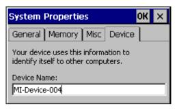
The «Device» tab displays the network name. The network name can also be set using <a href="Netsetup">Netsetup</a>. The device can be restarted if required after the network name is changed.
