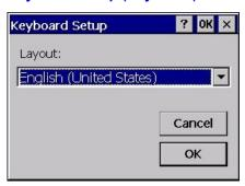
The keyboard setup – control panel makes the country setting for a USB keyboard. You can select the desired keyboard layout in the dialog shown above. The selected keyboard layout is still retained after a restart.
