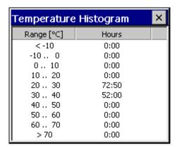
**Details** displays the total operating hours run, broken down into individual temperature ranges:
