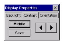
This program is used for setting the screen contrast. The «Middle» setting is the factory setting. Touch «Save» to save the selected setting as persistent data, i.e. the value is retained even after a restart.
