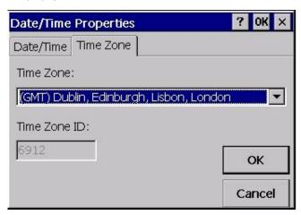
The dialog shown can also be used to set the required time zone. The «GMT» time zone is set by default, i.e. without a time shift setting. The set time zone is also retained after a restart.
