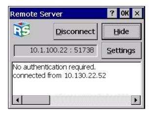
Touching the «**Hide**» button causes the dialog shown above to be hidden, i.e. only the icon start bar is visible. Use the «**Disconnect**» button to close the current client/server connection. The «**Password Settings**» button can be used to modify the password settings.
