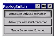
The «Repllogswitch.exe» program is used for establishing a connection with a PC via «ActiveSync» or «Manual Server». This is described in the chapter <u>Procedure: ActiveSync</u> or <u>Procedure: Manual Server</u>.
