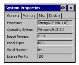
The «General» tab contains important information about the device and the installed Windows CE version. «Image Release» shows the version of the CE Image. See also the chapter\_Licensing.
