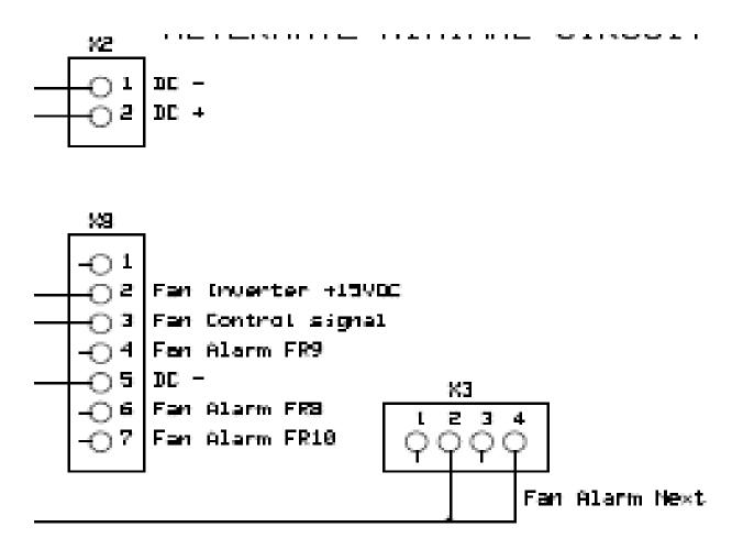
X2 pins 1 & 2 are DC bus. This comes from the DC bus of the drive through a pair of fast acting 6A fuses.
