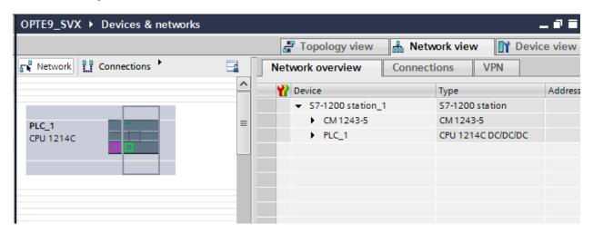
The PLC will be displayed. In the Catalog at the far right, select the arrow next to "Other field devices", then next to PROFIBUS DP / Drives / Vaasa Control/Vacon NX/Vacon NX. Drag and drop the device called Vacon NX below the controller/PROFINET master on the Network View screen. Then select the purple square on the PROFIBUS master and drag it to the purple square on the OPTC3 and release the mouse button. The following should now be displayed:
