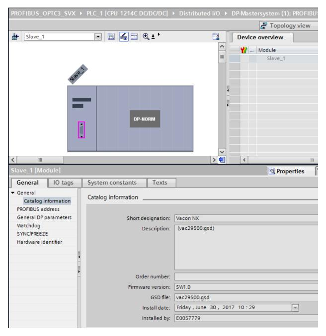
Select Profibus address on the left, then change the address to match the address selected for the OPTC3. Address 3 is used for this example.
