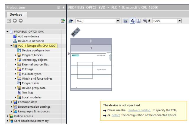
With the computer connected to the PLC via Ethernet, click the CPU box to select it, then select "detect" in the yellow area below it. The Hardware Detection screen will be displayed as follows:
