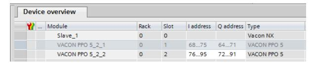
Note that the 'Vacon PPO 5\_2\_1' I/O addresses contain the Parameter Field data and the 'Vacon PPO 5\_2\_2' contains the Process Data Field I/O addresses.
