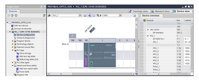
Select the PLC then click the Compile button. The compile button is just to the left of the Download button on the tool bar. Shown below are, from left to right: Compile button, download button and the upload button. As you hover over each of these buttons in the software, it will display its function.
