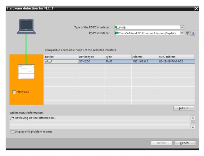
For this example, the Ethernet port on the computer is being used to communicate with the PLC. It will also be used to upload/download the project. Set up your computer and software to communicate with your PLC. Once communications is properly set up, select the Detect button and the software will detect the actual controller type as follows:
