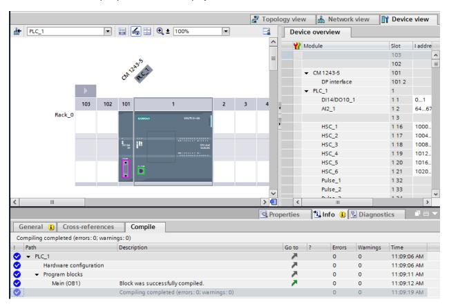
Next, select the download button to download the project to the PLC. The following window will be displayed. If the controller was in the Run mode, it must be stopped for the download. Select "Stop all" per the following, then select the Load button.
