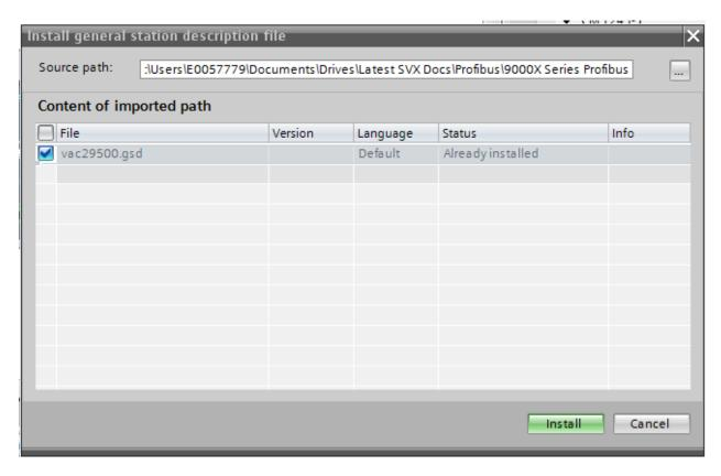
Select the 2 boxes by selecting the box next to File and next to the GSD file, then select Install and follow the directions to install the GSD file for the SVX drive.
