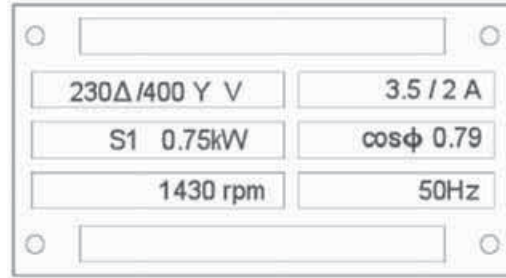
Figure 19. Example of a motor ratings plate
