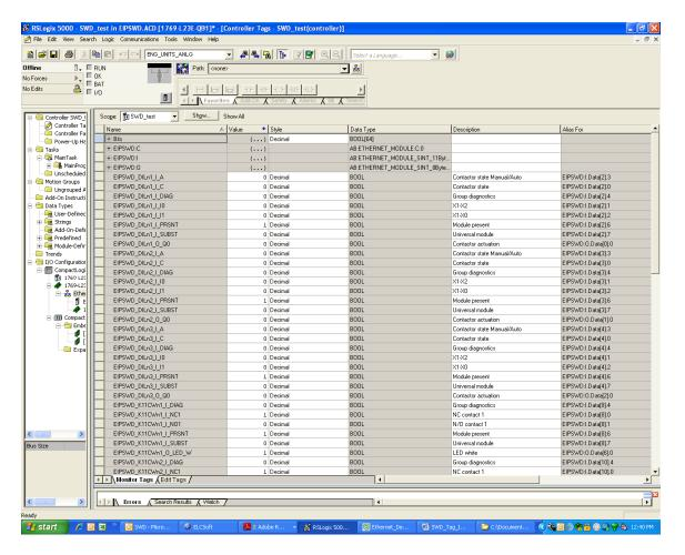
Note that all the tag names, descriptions and I/O addresses under the Name, Description and Alias columns exactly match the tag names, descriptions and I/O addresses in the SWD-Assist project.
