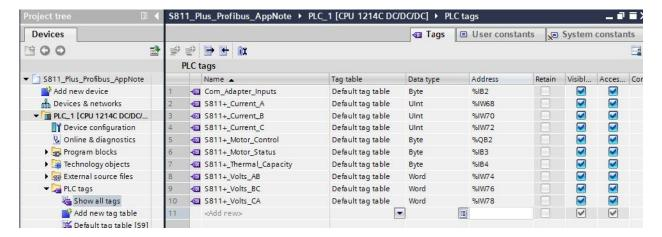
For the purposes of this application example, these tags will be added to a Watch and Force table rather than a program to test controlling/monitoring the S811+ via the Siemens PLC and the Profibus network.
