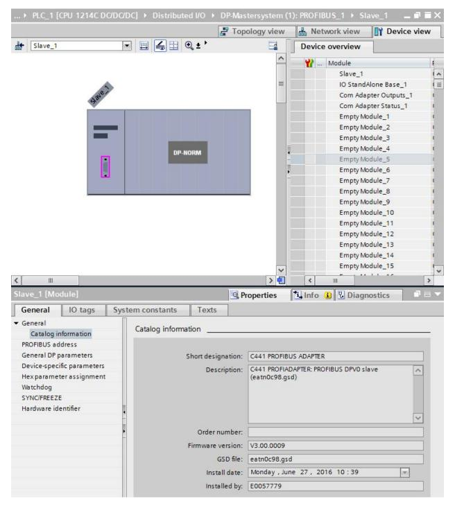
Change the Profibus address to match the address selected on the C441SS or C441QS. For this example, the Profibus address being used is 3. The Transmission speed will default to 1.5 Mbps, which is fine. Any speed will work here because the C441QS and C441SS modules auto detect the data rate from the master. The data rate is dependent on the overall network cable length.
