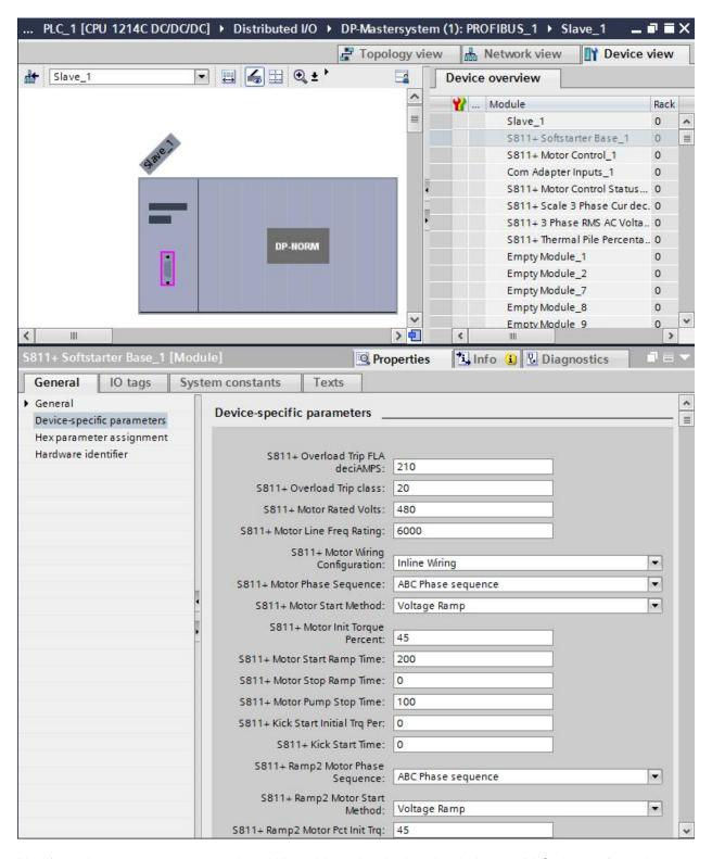
Modify each parameter as appropriate. When this project is downloaded to the PLC, the configuration files for each device will also be downloaded. These files, if enabled to do so, will then be downloaded to each slave device each time the master establishes a connection with them.
