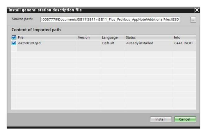
Select the 2 boxes by selecting the box next to File and next to the S811+ GSD file, then select Install and follow the directions to install the GSD file for the S811+ Soft Starter.
