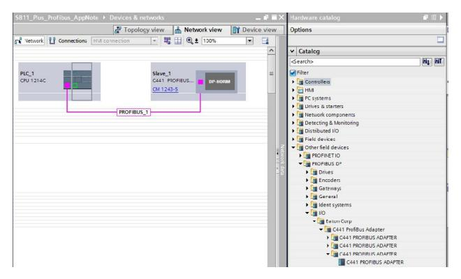
The Profibus network has been created in the offline project. Double click the Slave\_1 C441 Profibus module and the following will be displayed:
