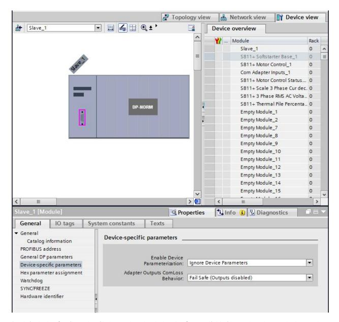
By default, the Configuration file is not downloaded to the S811+. If this feature is to be used, change the Enable Device Parameterization selection above to Download Device Parameters.
