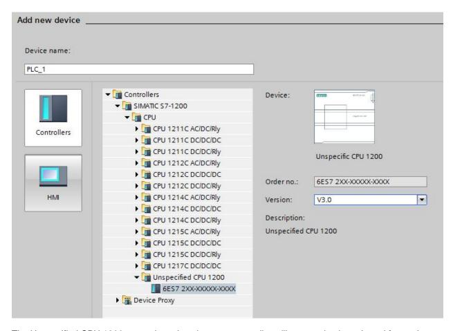
The Unspecified CPU 1200 was selected so the exact controller will not need to be selected from a long list of controllers. This selection will allow the software to auto detect the controller, as demonstrated below.
