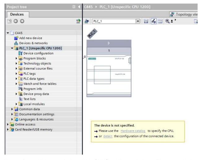
You must first establish communications with the CPU. Since this controller has an Ethernet port, that is the port used in this example to communicate with the CPU.
