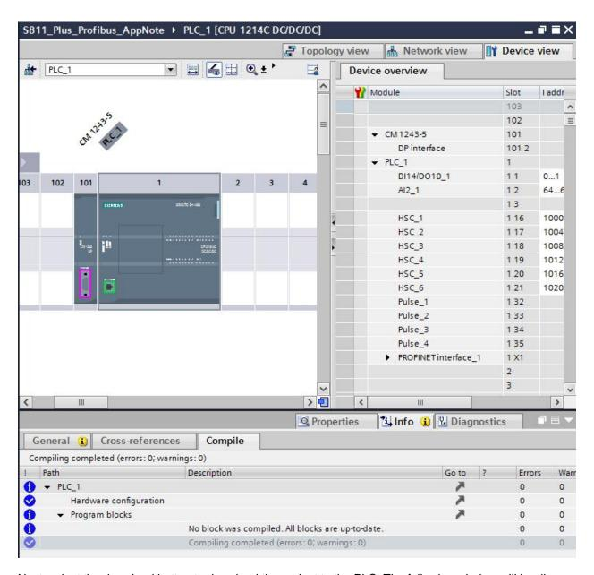
Next, select the download button to download the project to the PLC. The following window will be displayed. If the controller was in the Run mode, it must be stopped for the download. Select "Stop all" per the following, then select the Load button.
