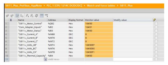
The S811+ can be configured for either 2-wire or 3-wire control, with 3-wire control as the default. The C441 Profibus modules sense the mode the S811+ is configured for and writes control information to the appropriate control register in the S811+. It's important to note the difference between the 2-wire and 3-wire control bytes.
