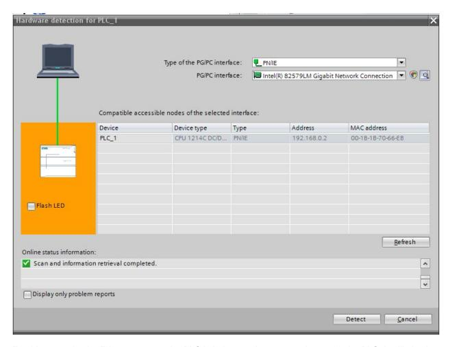
For this example, the Ethernet port on the PLC is being used to communicate with the PLC. It will also be used to upload/download the project later. Set up your computer and software to communicate with your PLC. Once communications is properly set up, select the Detect button and the software will detect the actual controller type and the Profibus master module connected to it as follows:
