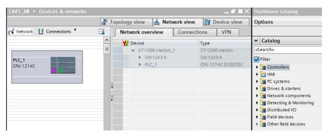
The PLC will be displayed. In the Catalog at the far right, select the arrow next to "Other field devices", then next to Profibus DP / I/O / Eaton Corp / C441 PROFIBUS Adapter / C441 Profibus Adapter. Drag and drop the device called C441 Profibus Adapter below the controller/PROFIBUS master on the Network View screen. Then select the purple square on the PROFIBUS master and drag it to the purple square on the C441 module and release the mouse button. The following should now be displayed:
