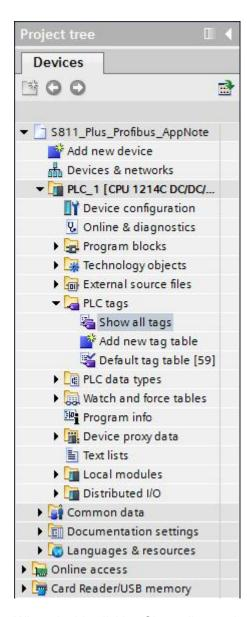
When double clicking Show all tags, the PLC tags screen will be displayed. Add tags to this screen as shown below. Names are entered for each tag and these tag names can then be used in the user program.
