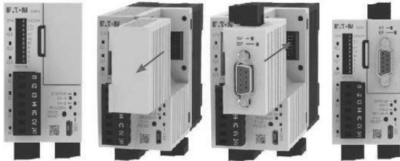
Figure 133. Installing the PROFIBUS Communication Card
